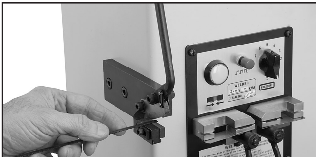
Figure 26. Using the blade shear to cut the blade.
